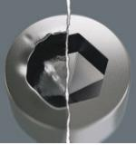
Hexagon screws can endure a problem because the contact surfaces delivering the power from conventional the tool, is transferred to the screw via very small surface areas. The consequence: the screw can become damaged (rounding out). Hex-Plus tools have a greater contact surface that prevents this from happening! At the same time, as much as 20 % more torque can be applied. Good to know: Hex-Plus tools fit into every standard hexagon socket screw!
